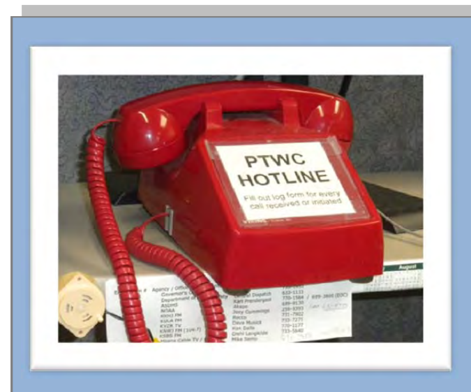
Figure 3.3 - Direct phone line between the Pago Pago Weather Service Office and PTWC for tsunami warnings. (EA/HHF, 2011)
